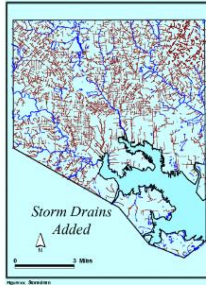
FIGURE 3-18 Baltimore City before and after development of its stormwater system. The left-hand panel shows first- and second-order streams lost to development. The right-hand panel shows the increase in drainage density resulting from construction of the modern storm-drain network. SOURCE: Courtesy of William Stack, Baltimore Department of Public Works.
